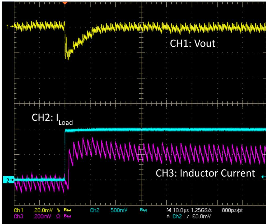
**Figure 4: Transient Response with Gain Setting = 650 (Bandwidth = 70kHz)**
