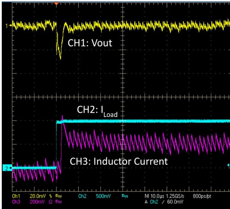
Figure 5: Transient Response with Gain Setting = 1050 (Bandwidth = 140kHz)
