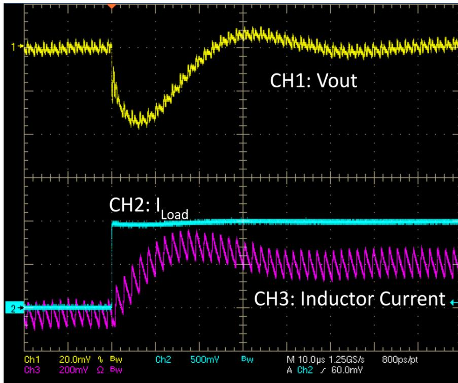
Figure 3: Transient Response with Gain Setting = 250 (Bandwidth = 26kHz)
