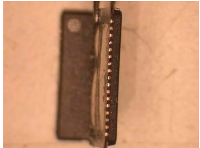
FIGURE 17. FINISHED TINNED THERMAL LAND ON QFN
