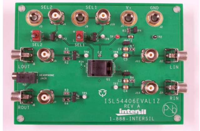
FIGURE 1. ISL54406EVAL1Z EVALUATION BOARD
