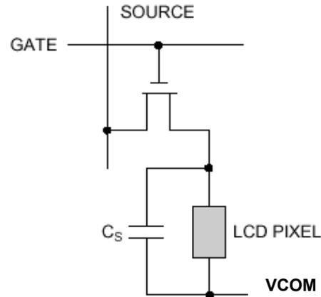
**FIGURE 2. CIRCUIT DIAGRAM FOR SINGLE LCD PIXEL**
