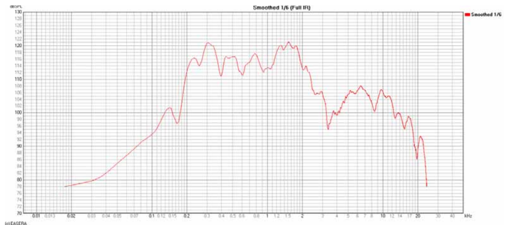
Typical Premium Digital TV Speaker Frequency Performance with 3.0” Driver
